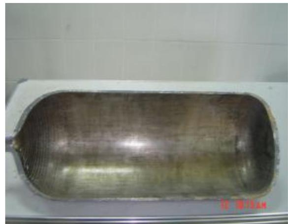
Cut Section of type 1 CNG Cylinder
