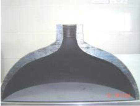
Cut Section of Type 1 CNG Cylinder Neck
